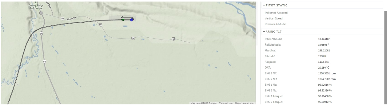
Fig. 6. Map and detailed information at a specific point in flight. Captured ARINC 717 data is presented here at the moment of takeoff.
